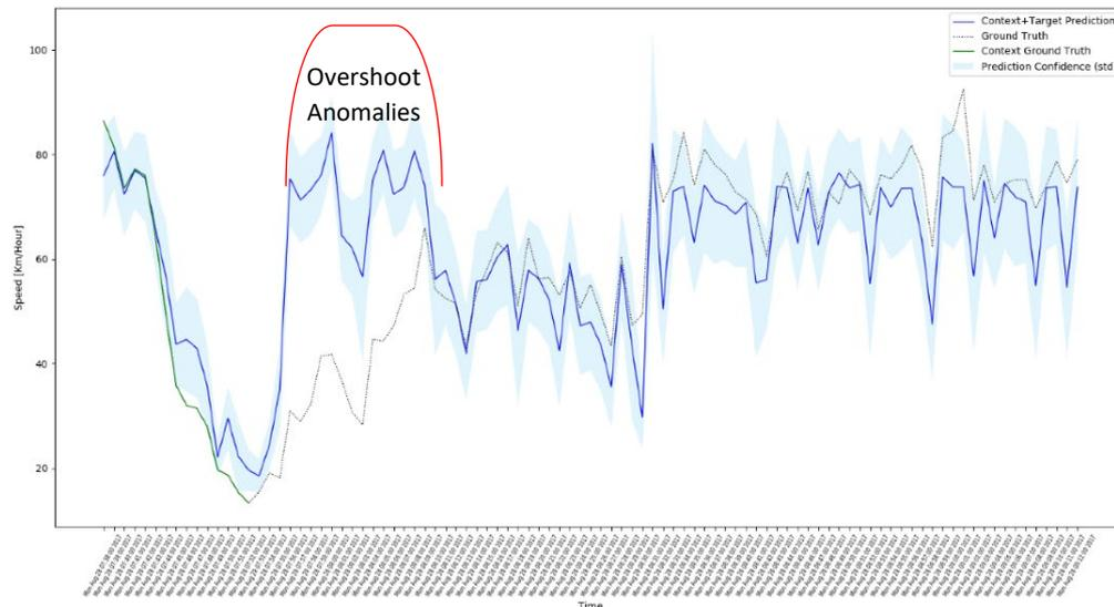
**Figure 2.** Automatic road incident detection and model generalization – the algorithm detects an incident (in red) caused by car accident along a testing freeway segment. The traffic slowdown afterward is reflected with consecutive set of overshoot anomalies. Moreover, it successfully models and predicts traffic flow on never-seen freeway segment data.
